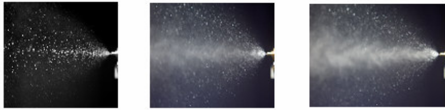
Figure 3. Development of spray with gas pressure at constant liquid pressure
